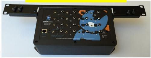
4. Attach assembly within 19" rack. (AudioFetch rails + enclosure = 4U spacing.)
